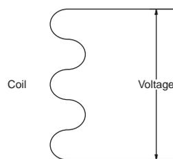
For proper valve operation, power to the coil should be controlled with a double pole switch
