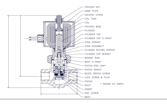
Shown is a Model 31830 3/4" Stainless Steel Valve with an AC Coil & NEMA 1 Coil Housing
