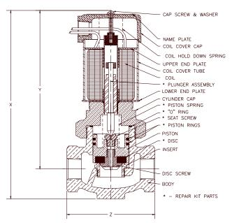
Shown is a Model 4400 a 1" Bronze Valve with a Standard NEMA 1 Coil Housing
