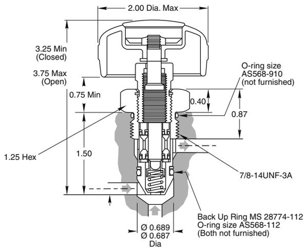
C900 Series—inlet size 0.203, outlet size 0.250. O-ring seals for manifold cavity are furnished by customer.
