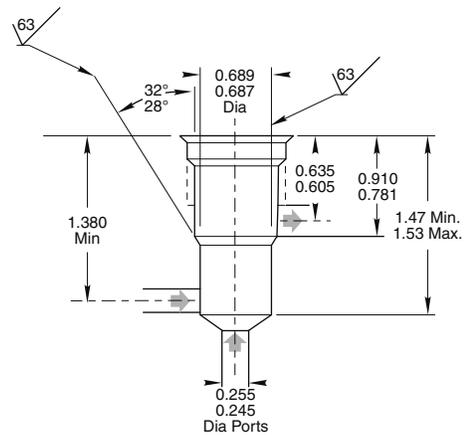
Cavity per AND10050-10 or SAE ½" straight thread connection (½-14UNF-3B) except as shown.
