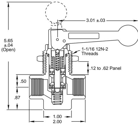
Spring and ball detent positively position handle open or closed. Holes are provided in toggle cam and clevis to permit locking valve closed against tampering.
